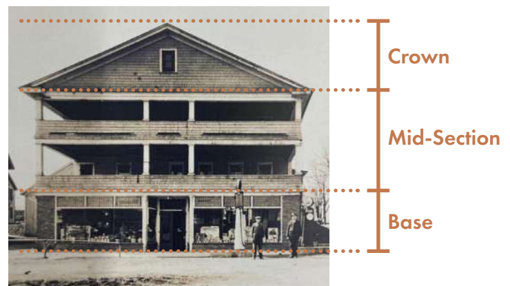
The hotel at the Four Corners exhibits a traditional tripartite façade design.
